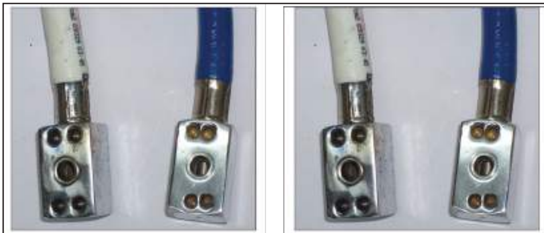
Figure 5 & 6: Non interchangeable screw threaded system for various gases (These other end of flexible hose are connected on anaesthesia machine)
