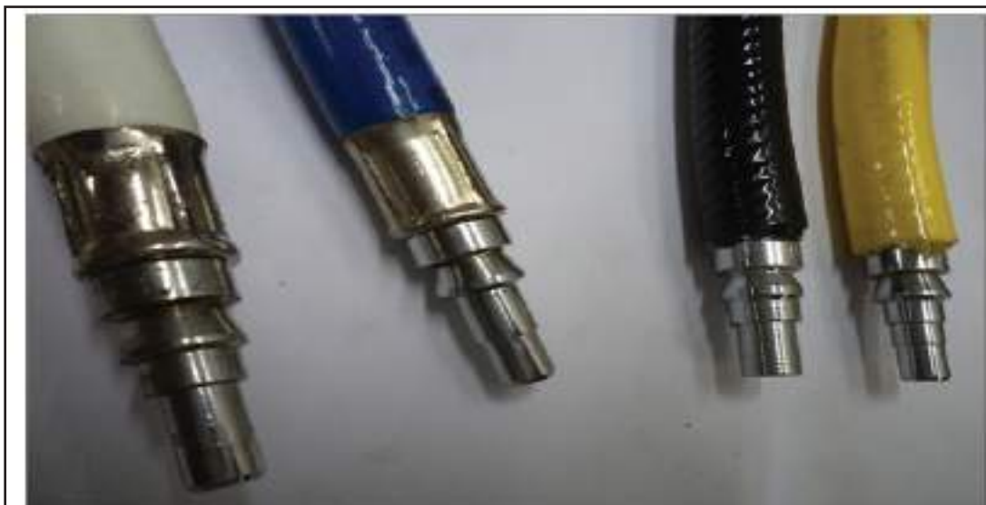
Figure 4 – Schrader probes for different gases from flexible hose pipelines (Connected to the terminal wall outlets)
